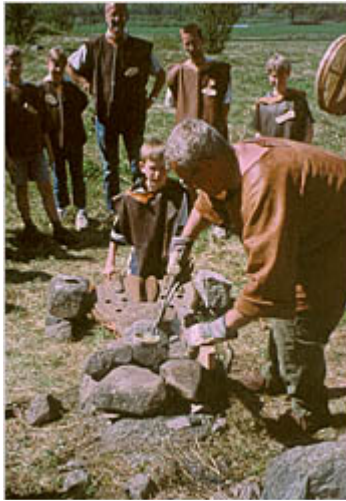
Here we pour the melted bronze into the mould.
